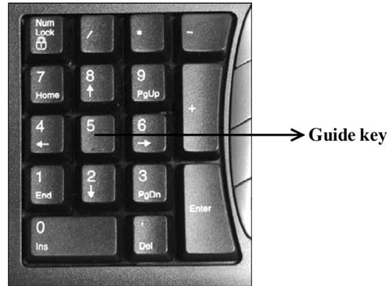
**Fig. 3.10 : Guide key on Numeric keypad**
